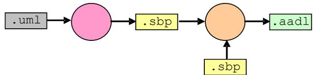
The work-flow now consists in parsing the XML file representing the UML MARTE model. This parsing is achieved by xmlrev, another tool from the LMP toolbox that works in a similar way as aadrev excepts that it produces a fact base describing the structure of an input XML file:
