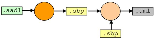
The work-flow consists in parsing the textual AADL specification with aadrev (orange circle), then to apply the resulting facts base and the transformation rules base to the sbprolog engine (pink circle). The transformation rules must include in that case the AADL – MARTE mapping as well as an XML generator complying with the UML meta-model.
