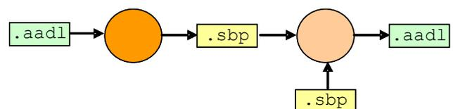
The work-flow associated with such homogeneous transformations is as shown above, where the orange circle represents the aadrev parser and the pink circle the sbprolog engine.
