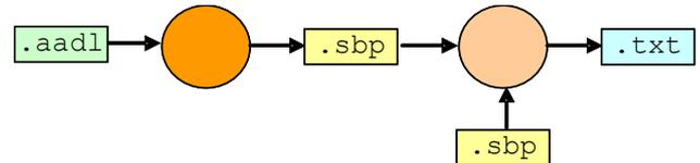
The work-flow is now enriched with a second processing segment where the pink circle represents the sbprolog engine that takes the byte code facts base and the byte code rules base as input and produces a textual report.
