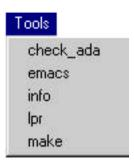
The *tools* menu is a fully customizable. Each item refers to a shell script file located inside <code>config/externalTools</code> configuration directory. Proposed items may be removed or modified, and others may easily be added to the list. Each file should have a .sh suffix to be automatically included into *tools* menu items list
